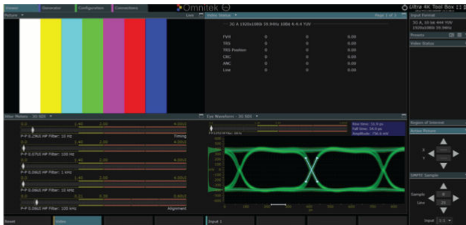
Figure 7. Video Image and Jitter Result for Video Format 1920 x 1080i 59.94 Hz
