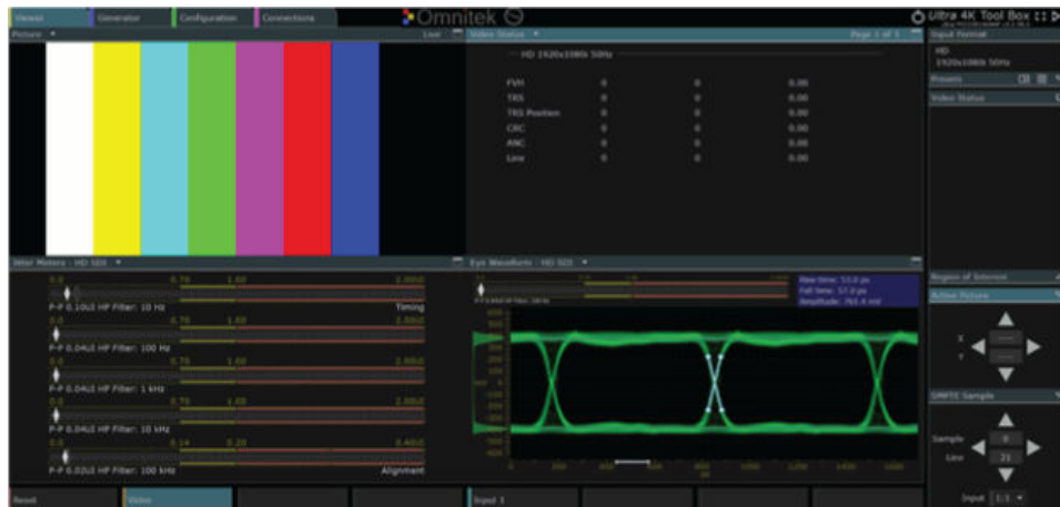
Figure 9. Video Image and Jitter Result for Video Format 1280 x 720p 29.97 Hz
